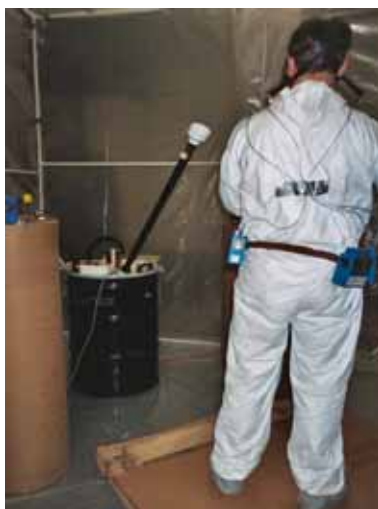
Photograph 3. 5: Feeding Bulbs into the Manufacturer C Device
